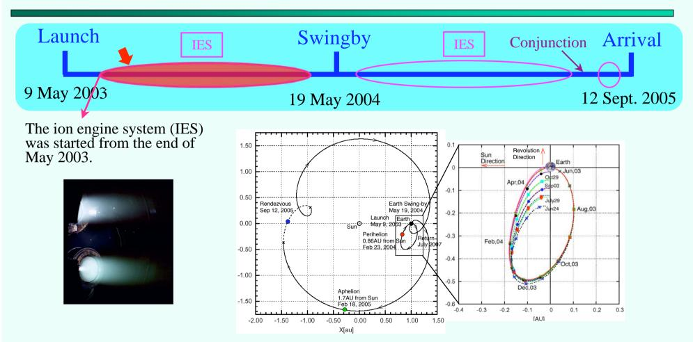
The Orbit determination under the thrust of the ion engine is difficult, so we made "ballistic period" (=ion engine is stopped) of about three days once in a month, and performed the orbit determination.
