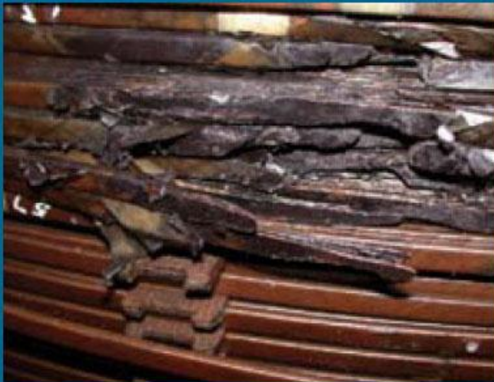
Failure in a large South African generator transformer, three weeks after the Halloween storm of 2003.
