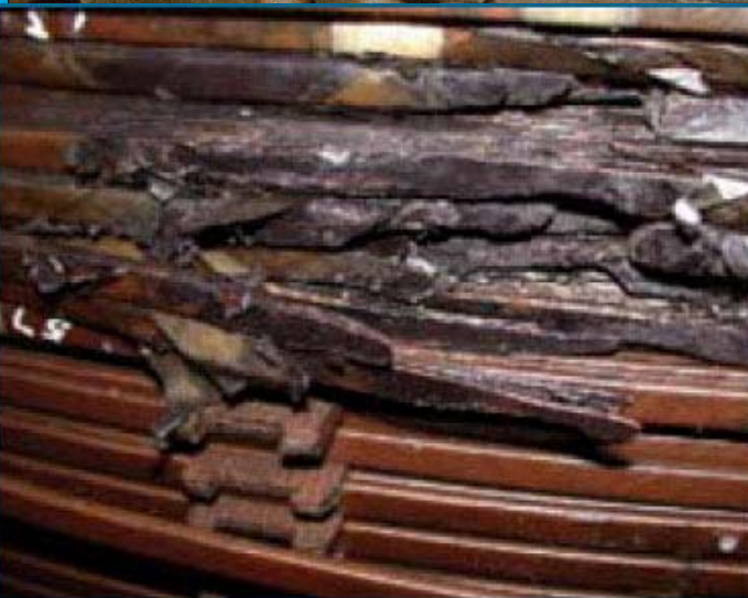
Failure in a large South African generator transformer, three weeks after the Halloween storm of 2003.
